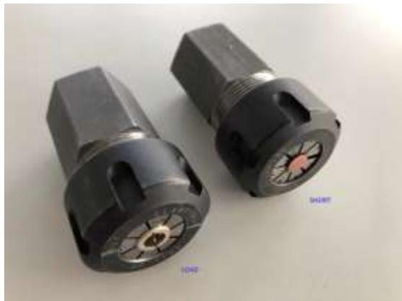
The calibration kit contains of a thru, a load and a short artefact.
