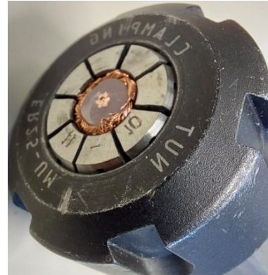
Figure 5: Folded screen preparation and cable end face after installation in cable holder
