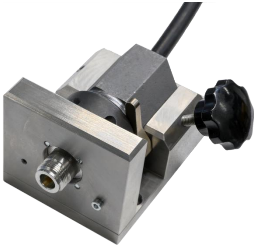
Figure 7: The universal connector (with N interface) with cable in place
