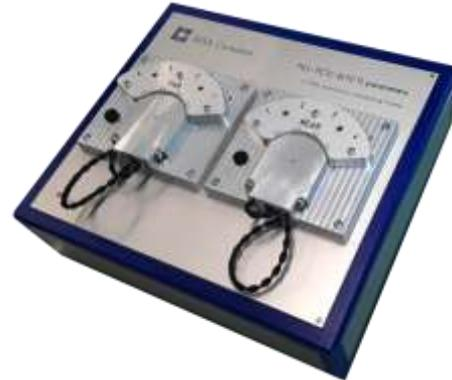
*Fixture for U/FTP, F/FTP and S/FTP cables*
