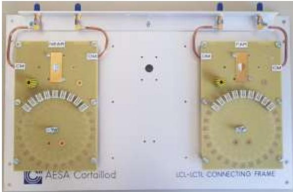
*Fixture for U/UTP, F/UTP and SF/UTP cables*
