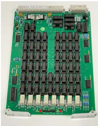
LF switching board “AZU” [55.0205.0119.0]:
