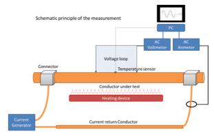
Although similarities can be found with DC linear resistance measurements, such as an adequate electrical connection of the conductor to achieve steady current distribution, additional specific considerations are necessary for an accurate AC measurement, i.e.:
