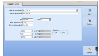
2. **Specification measurement**: The operator preselects a specification (created previously by a supervisor). Graphical information is also available. It is possible to select previous measurement and to print the last value measured.
