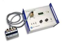
The **HV DC generator 4735** performs dielectric strength with adjustable voltage without destruction of the cable in the event of a breakdown. The low supplied current (0,3mA) prevents the destruction of the cable in case of default. The fault is indicated by the variable lighting of the lamp, flashing when the current leakage reaches  $10\mu A$ .
