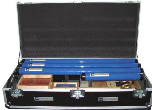
This option allows measuring the transfer impedance, the shield attenuation and the coupling attenuation when knowing the impedance of the internal coaxial cable created with the sample under test. This impedance can be keyed in our software to perform then the different required calculations.
