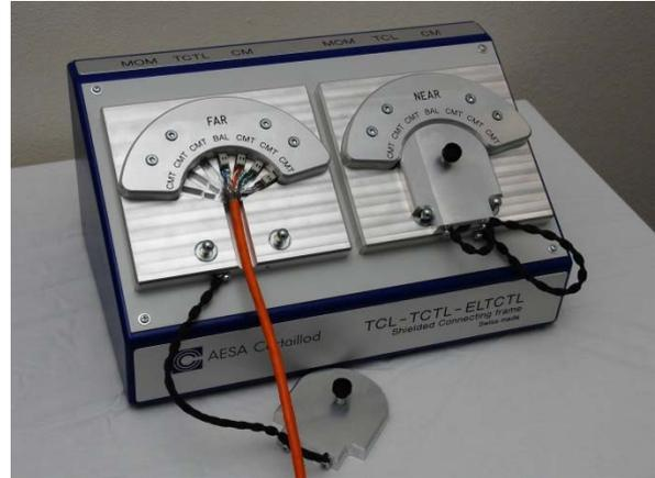
*Fixture for U/FTP, F/FTP and S/FTP cables*
