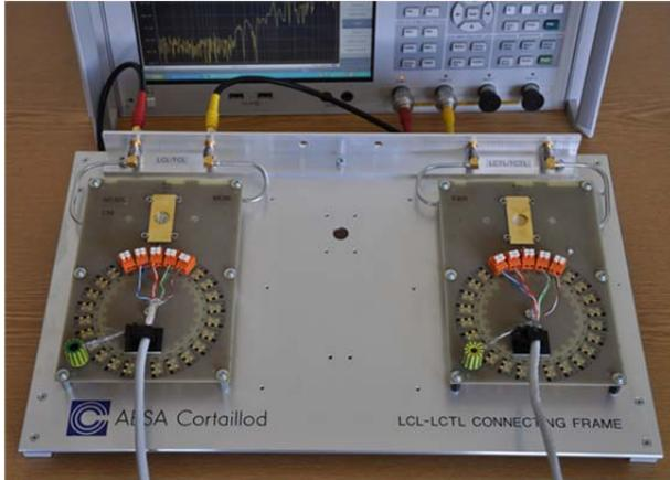
*Fixture for U/UTP, F/UTP and SF/UTP cables*
