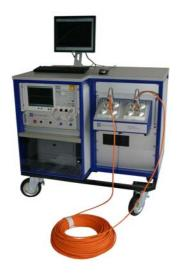
For convenience or operational reasons, it is possible to add a professional movable trolley to the system. In such a case, all tester components are integrated in the trolley, including the computer system and the printer.
