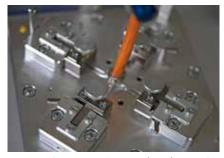
Automatic test equipment (ATE) must be used to perform these numerous tests that not only provide "Pass" or "Fail" information but also the complete cable characterization profile.
