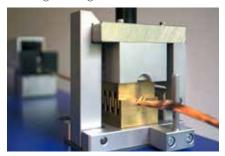
The AESA ResTest family consists of integrated equipment specifically designed for the cable industry. These resistance bridges not only offer operating comfort, but also allow you to master all related uncertainties (temperature, length, current distribution,...) to ensure full reliability of the measurement.
