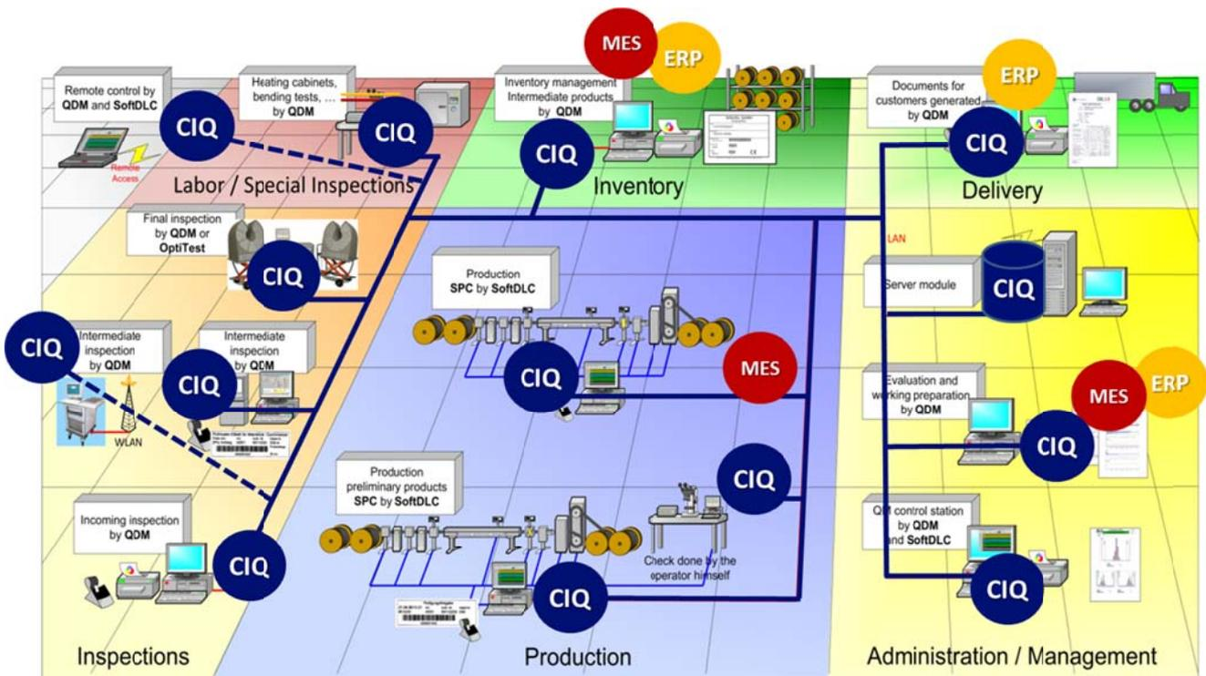
**Figure 4. The roles of CIQ as well as ERP and MES within the factory floor**
