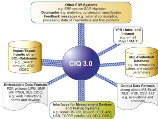
Figure 2. Interfacing and integration of the CIQ within IT infrastructure
