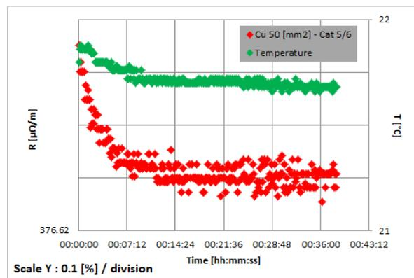
Fig 2 Resistance and temperature courses during stabilization.
