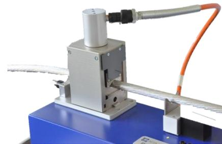
Fig 6. Hydraulic clamping block
