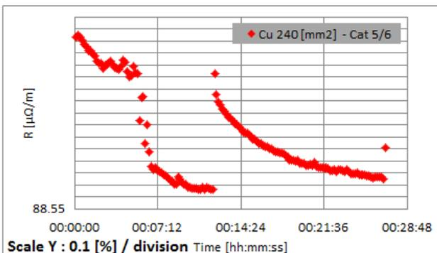
Fig 4. Instabilities in measurements due to inter-wires contact resistance
