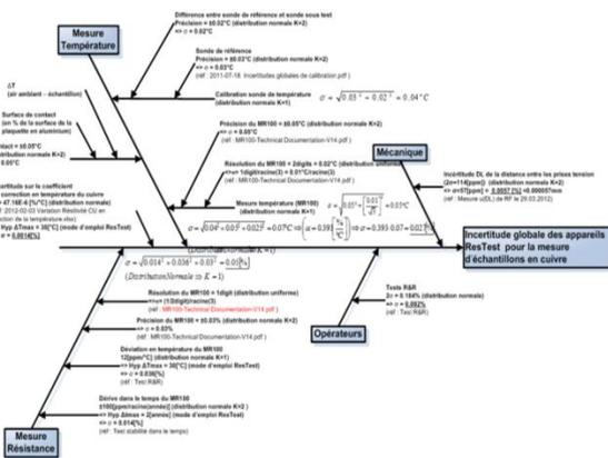
Fig 1 Ishikawa diagram for the analysis of uncertainties by testing copper samples
