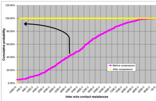
Fig 3. The contact resistance depends strongly on applied pressure
