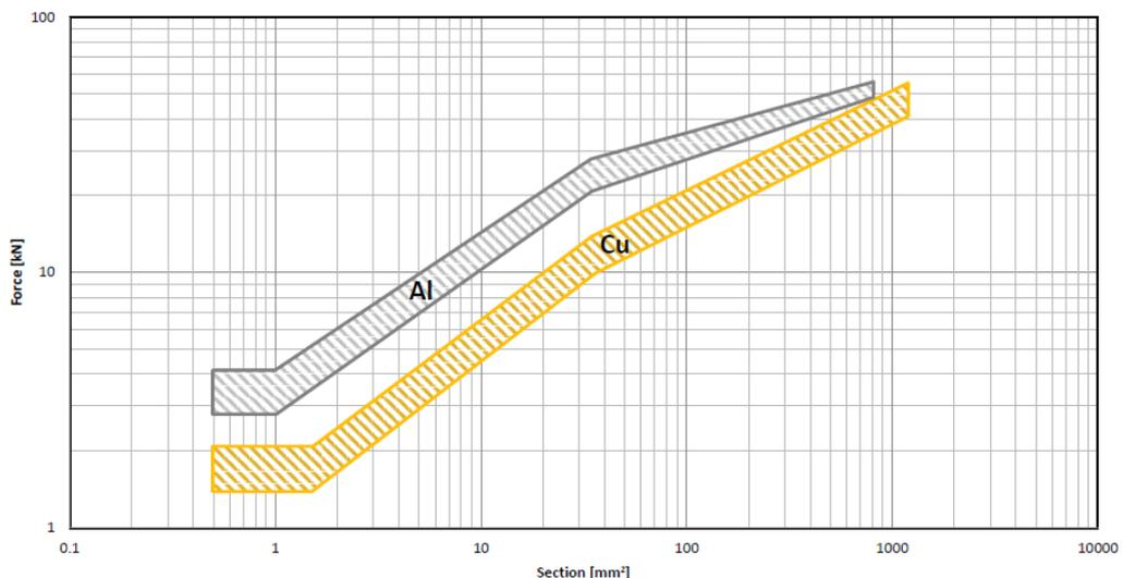
Fig.12: Attempt of recommended clamping force in function of section and material
