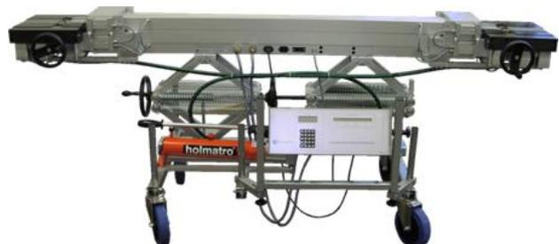
Fig 8. AESA 8135 "on-the-line" Resistance & cross-section measurer
