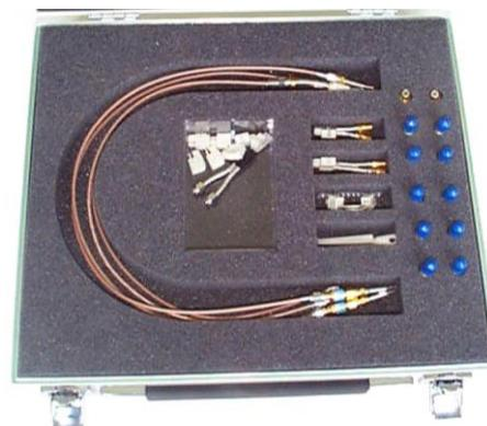
During a quality control, the symmetric artifacts have to be replaced by  $50\Omega$  certified coaxial standards. Using an appropriate set of terminations and attenuators, it is possible to prove within a given tolerance that the system (network analyzer + HF multiplexer + connecting frame) is measuring correctly. It is also possible to prove that the calibration used for the measurement of LAN cables has been done properly.
