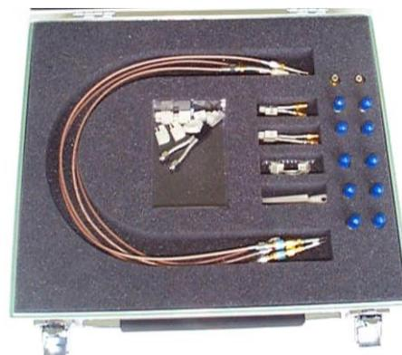
During a quality control calibration, the symmetric elements have to be replaced by 50 $\Omega$  coaxial standards which are this time certified. In fact, with an appropriate set of terminations and attenuators, it is possible to prove within a certain tolerance that our VEGA system (network analyzer + HF multiplexer
