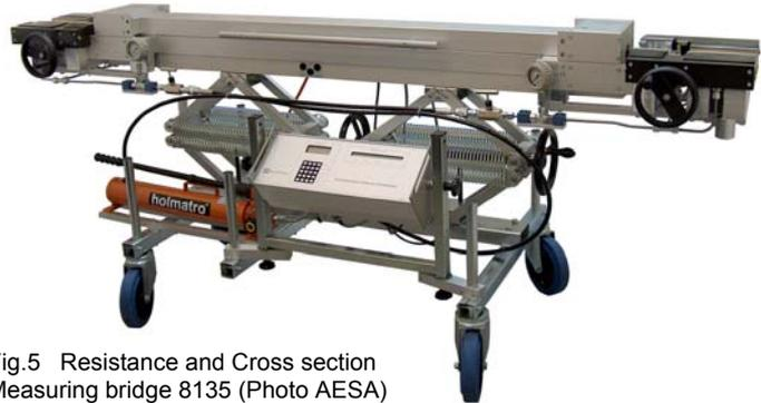
Fig.5 Resistance and Cross section Measuring bridge 8135 (Photo AESA)
