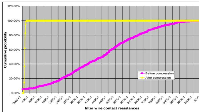
Fig. 6 Statistical distribution of contact resistances
