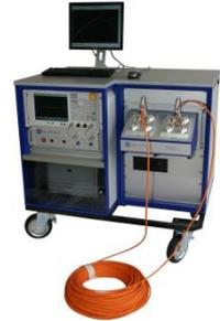
*Fig.9: AESA Vega 2004 HF automatic measuring equipment*
